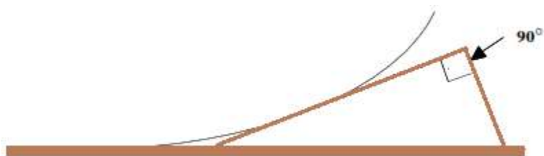
Correctly positioned wooden wedge
