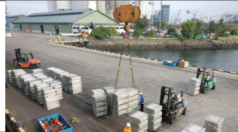
Handling of unbundled heavy T-ingots at Jurong Port with the use of a chain sling.
