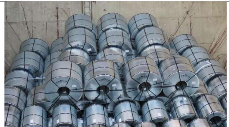
Pyramid stow of CRCs with a third tier of coils with good lashing. The heavy coils are not on top of the lighter ones.
