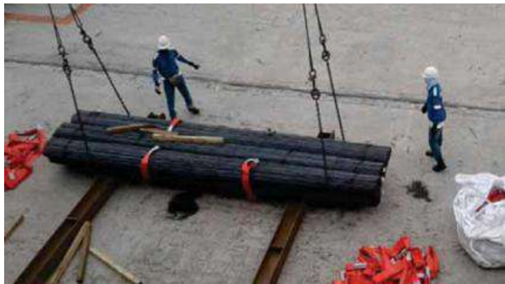
Pre-slung 6 m long bundles about to be loaded. Pre-slinging reduces the time needed for discharge operations.
