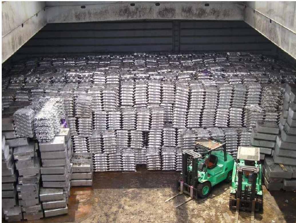
Small-size bundled ingots and T-ingots being handled, by a forklift truck, from the wing space.
