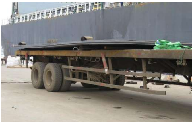
Unbundled, long steel plates.
