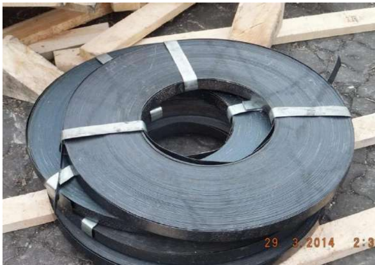
Metal strapping used for securing of pipes. The tightening should be made with the use of pneumatic tools.
