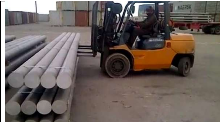
Bundled, long round aluminium billets handled with forklift truck and prepared for loading.
