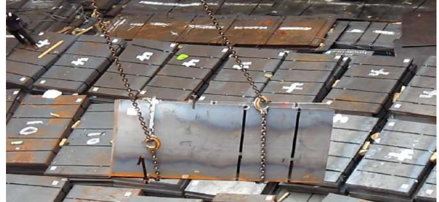
Bundled steel plates. Broken steel straps. Incorrect choke hitch application.
