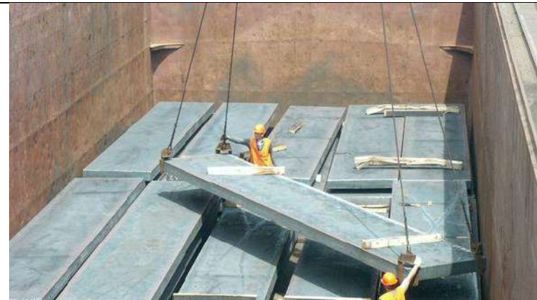
Loading of slabs in progress. Good, square, hardwood dunnage is used between the tiers.
