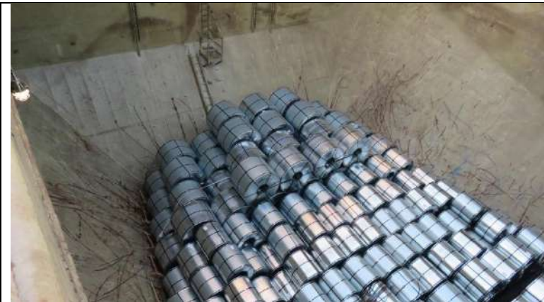
A good pyramid stow of CRCs in the aftmost part of a hopper-type cargo hold.
