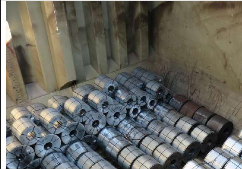
Locking coils or chocking dunnage must be placed on the first-tier coils in the centre.
