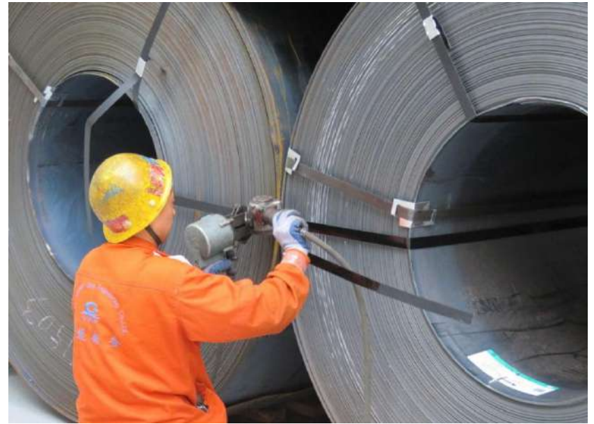
Tightening of steel strapping bands with a pneumatic tool. For coils of the size in the photograph, double metal straps should be used for lashing
