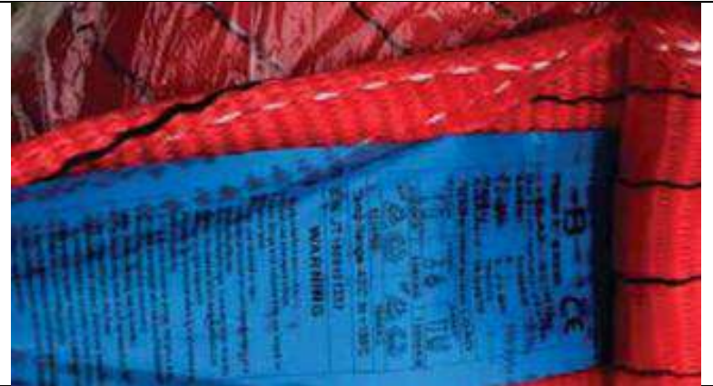
The slings for pre-slinging shall be certified and properly marked.
