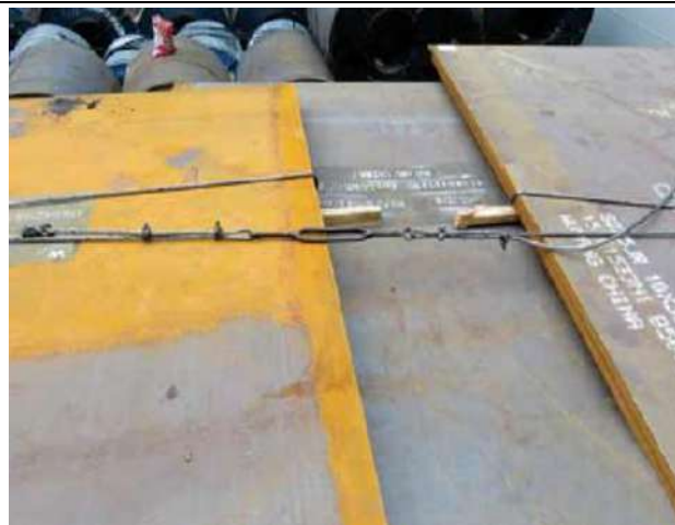
Incorrect use of bulldog grips with grips on the live wire. Insufficient number of grips used.
