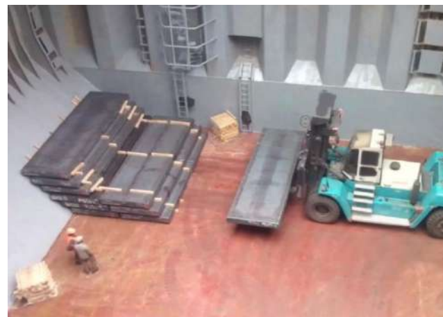
A fore-and-aft loading of slabs. Proper use of dunnage.
