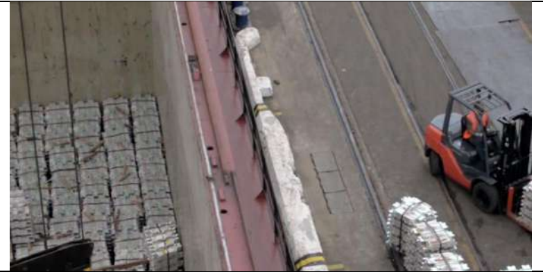
Box-type cargo compartment. Handling pre-slung, bundled medium-size ingots.
