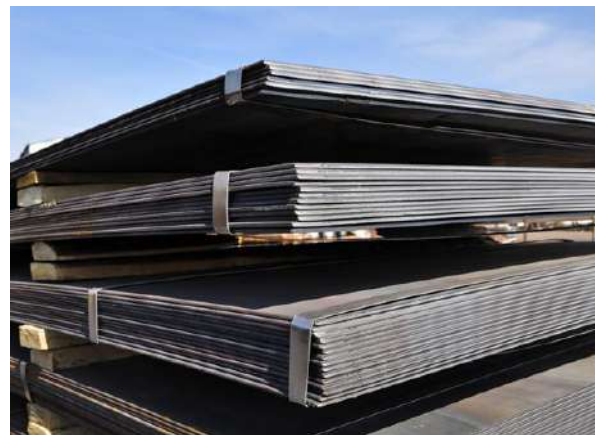
Bundled steel plates, ready for shipment. Only bundles of 110mm height are accepted for handling at Jurong Port.
