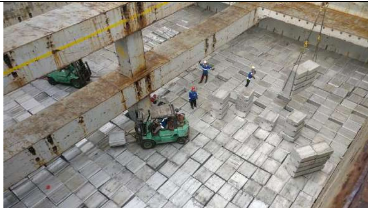
Jurong Port. The use of a forklift truck for the off-loading of T-ingots from a box-type cargo compartment. The stow is full and compact.
