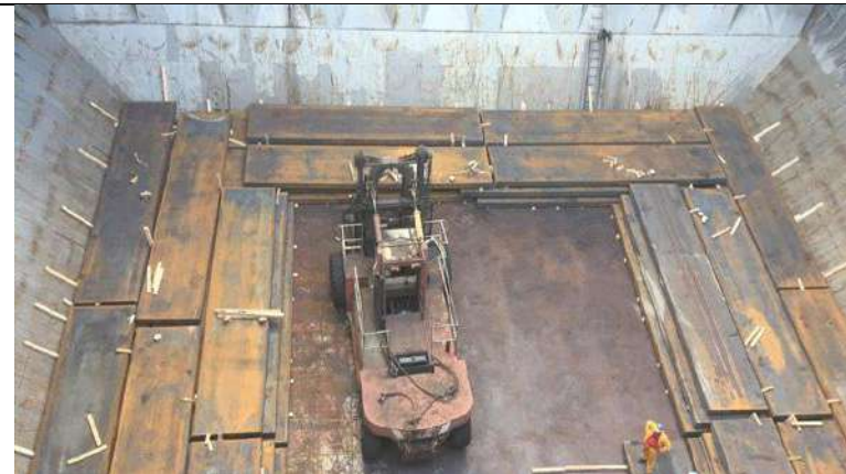
Loading and stowage of slabs in a hopper-type cargo hold. Proper dunnage should be used on the tank-top. The spacing should be a maximum of 2 metres.
