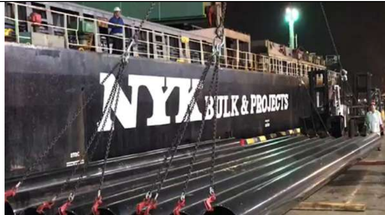
Pipe being discharged by pipe hook at Jurong Port.
