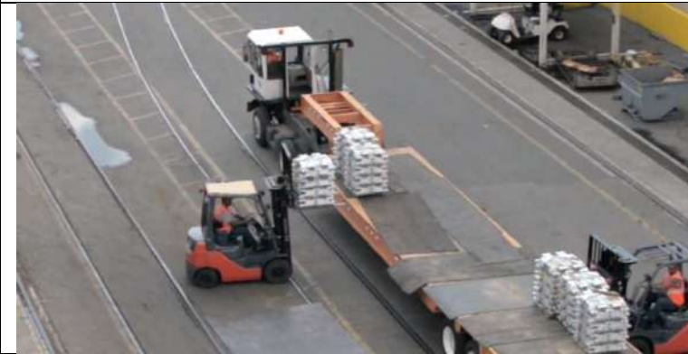
Handling pre-slung, bundled medium-size ingots. Loading on a trailer for further storage in a warehouse.
