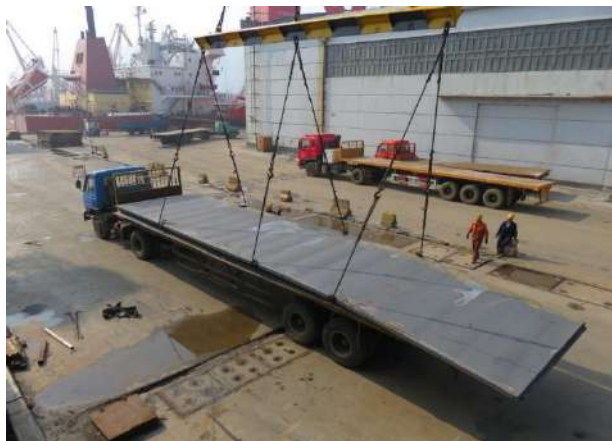
Unbundled, long steel plates loaded with a spreader.
