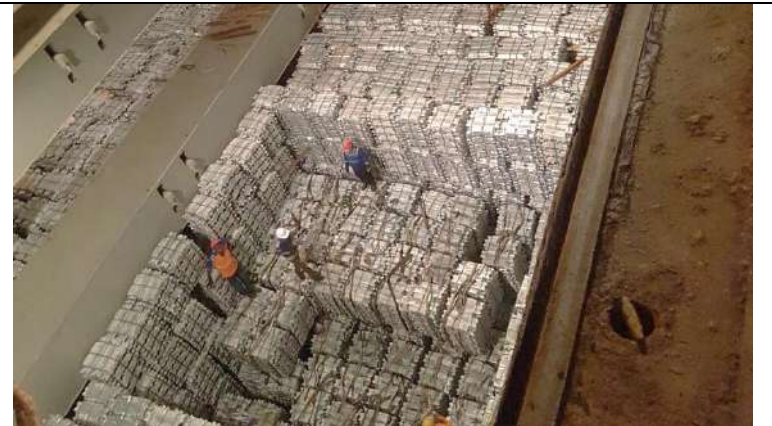
Jurong Port. Preparation of chain slings for off-loading of ingot bundles.
