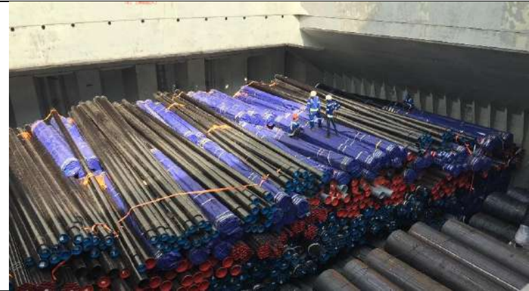
A loose stow of mixed size and bundled pipe, making discharge difficult, dangerous and slow. For mixed size pipes, pre-slinging is required.
