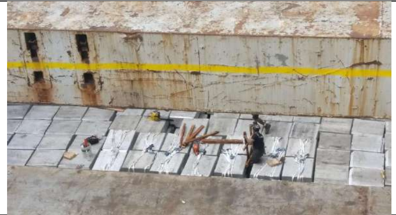
Jurong Port. Pre-slung T-ingots for first off-loading. Once the first units are removed, the remaining units are handled with a forklift truck.
