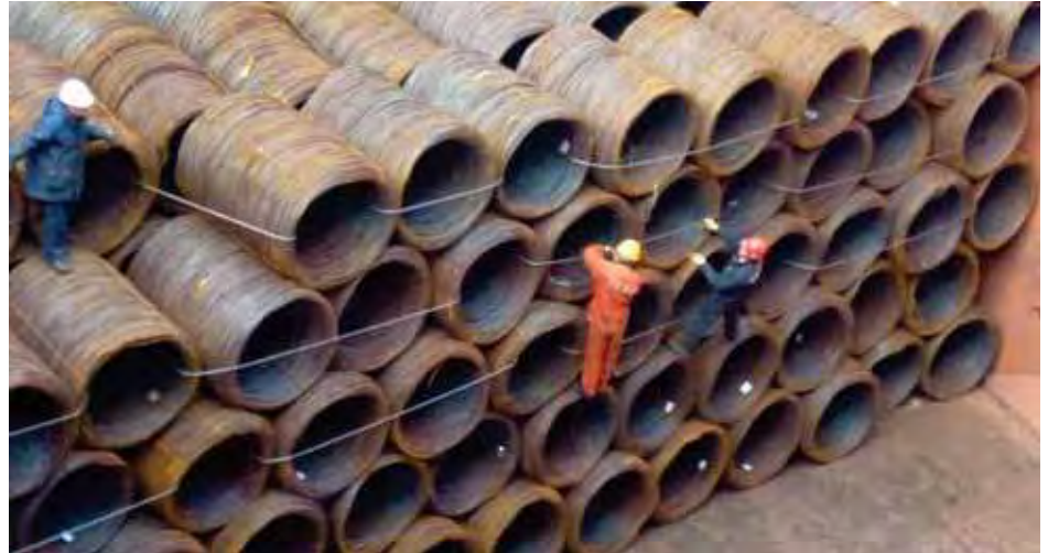
✘ Lashing the vertical face. Note the lack of safety harnesses. No safety access to the vertical part of the stow
