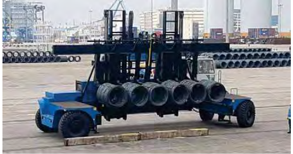
✔ Jurong Port has a multi-fork side-loader for transportation from the quay to the storage area
