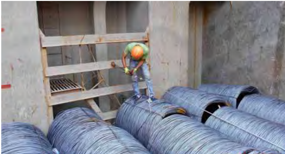
✓ The lashing wires are then secured to a designated lashing point inside the cargo compartment
