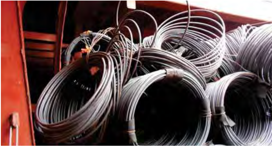
✘ Unwound and damaged coils. These should not have been loaded as they may be rejected by the receivers and will be difficult and dangerous to offload
