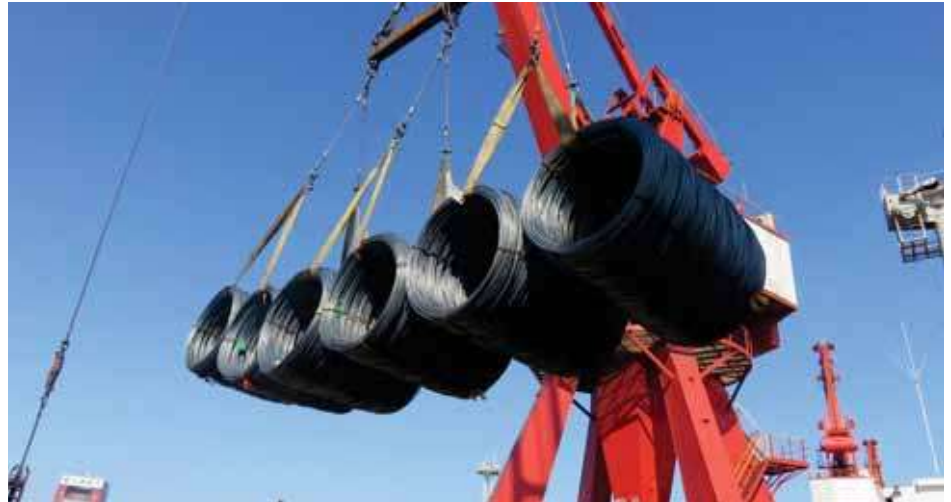
✔ By using lifting strops attached to beams (spreader), up to 6 coils at a time may be loaded in this layout
