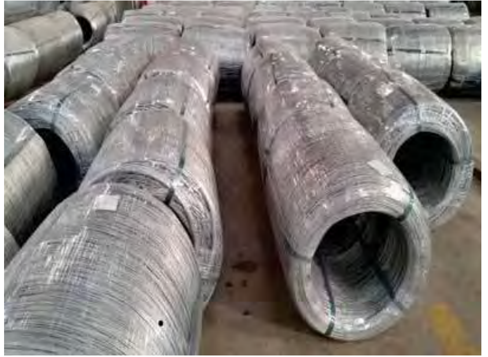
Partially protected WRIC secured with 4 strapping bands. The outer canvas/plastic cover offers some protection from the elements
