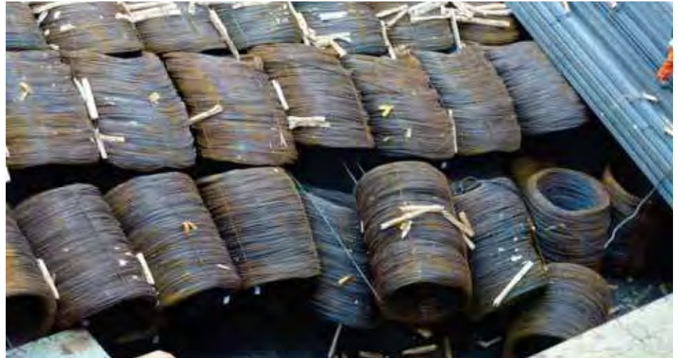
✘ Collapsed stow and deformed coils due to loading cargo above the coils
