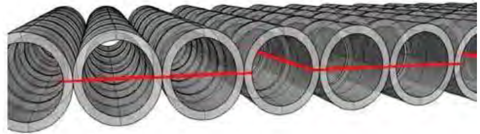
Lashing and securing arrangement of one tier of WRIC to the bulkhead (a view from the front)
