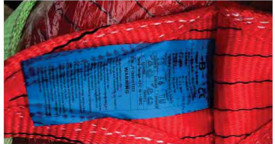
✔ The slings for pre-slinging shall be certified and properly marked
