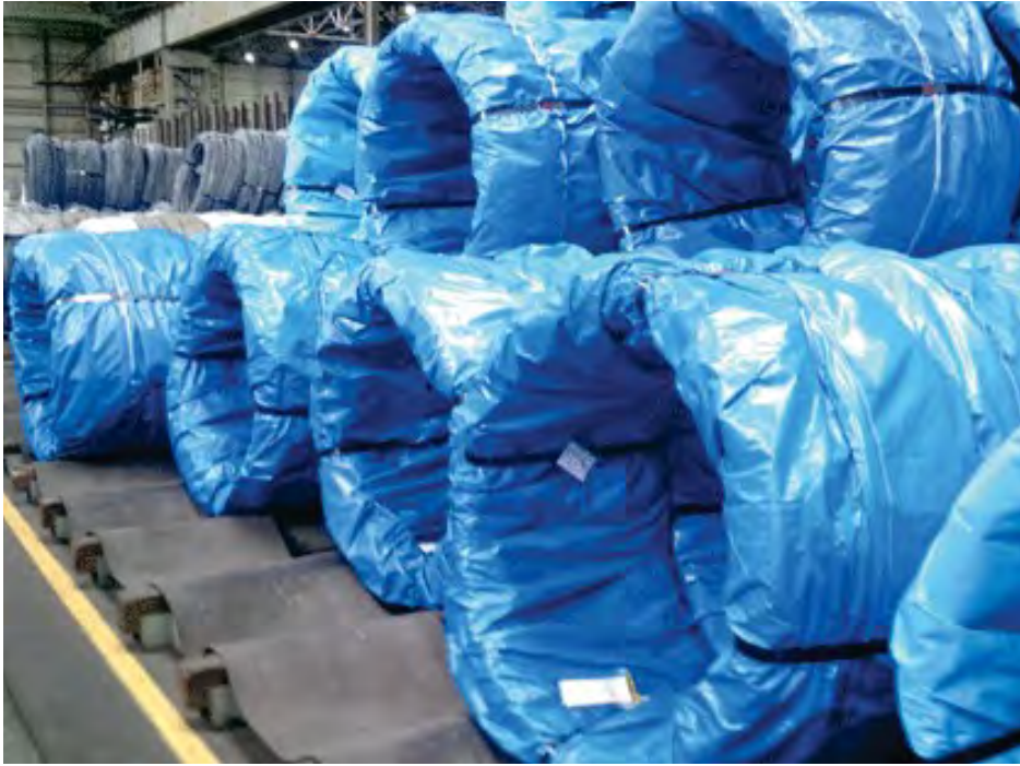
Partially protected WRIC secured with 4 strapping bands. The outer canvas/plastic cover offers some protection from the elements
