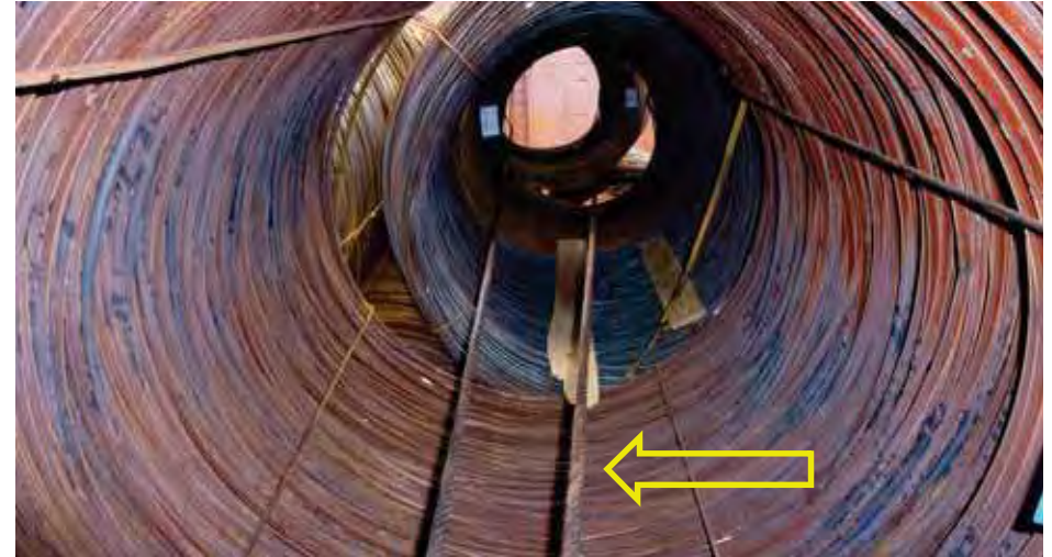
✓ The lashing wires are then passed through the coils towards the adjacent bulkhead
