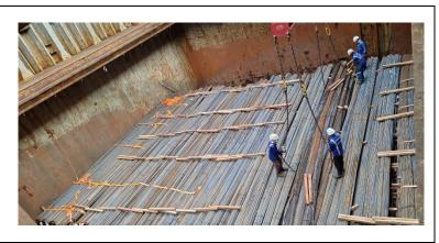
Recommended stowage of rebar in fore-aft direction. Dunnage laid out between tiers as shown.
