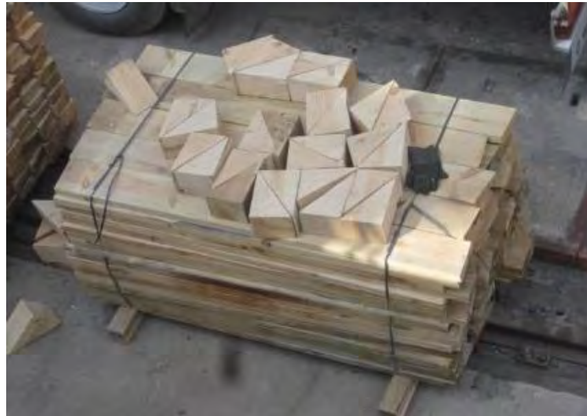
Dunnage boards and wood wedges prepared for the loading of steel coils.
