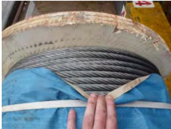
16mm wire rope supplied for lashing cargo.
