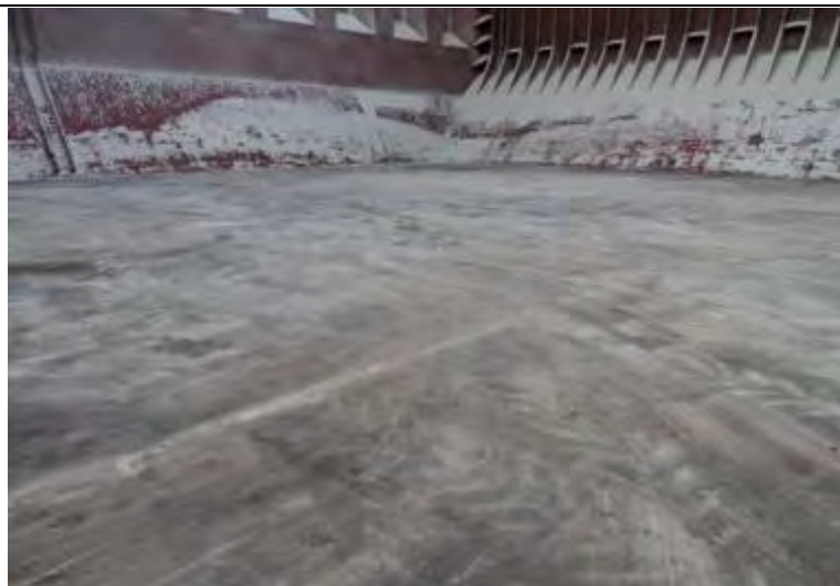
Poorly prepared cargo hold on a bulk carrier. Residue from some bulk cargoes can react with, and damage, the steel cargo.
