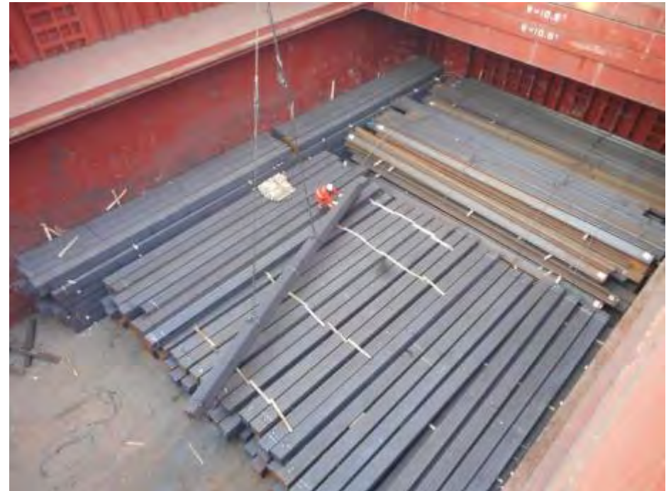
A good, even stow of structural steel bundles with dunnage between the tiers to assist the discharge operation.
