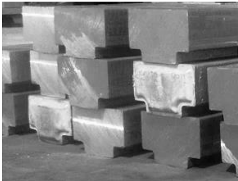
T-ingots vary in weight from 500kg upward and handled individually.
