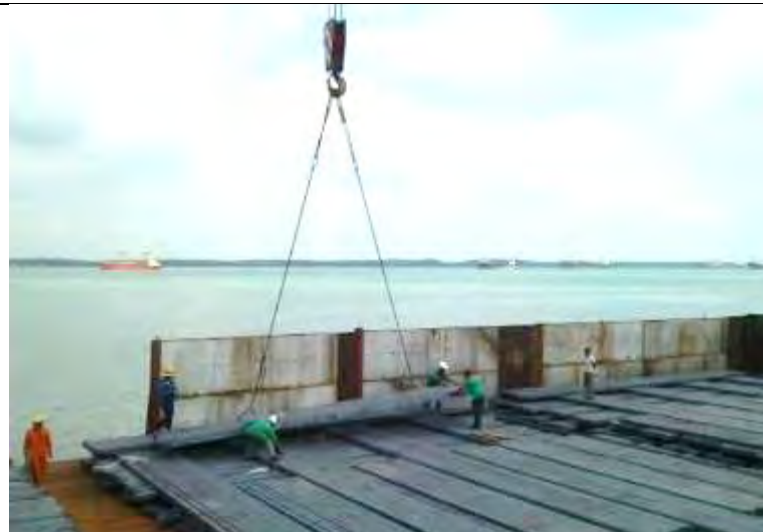
Off-loading billets with the use of a choke hitch.
