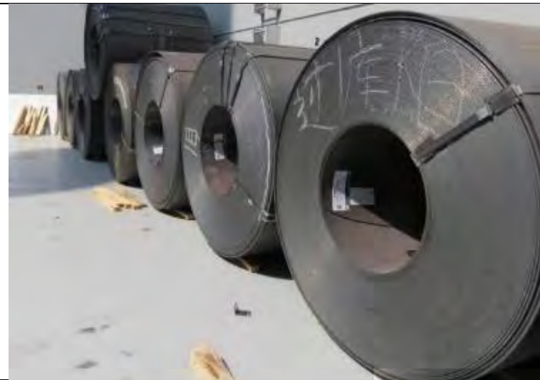
The HRCs have irregular and insufficient transverse metal straps. Such coils shall not be accepted for loading.
