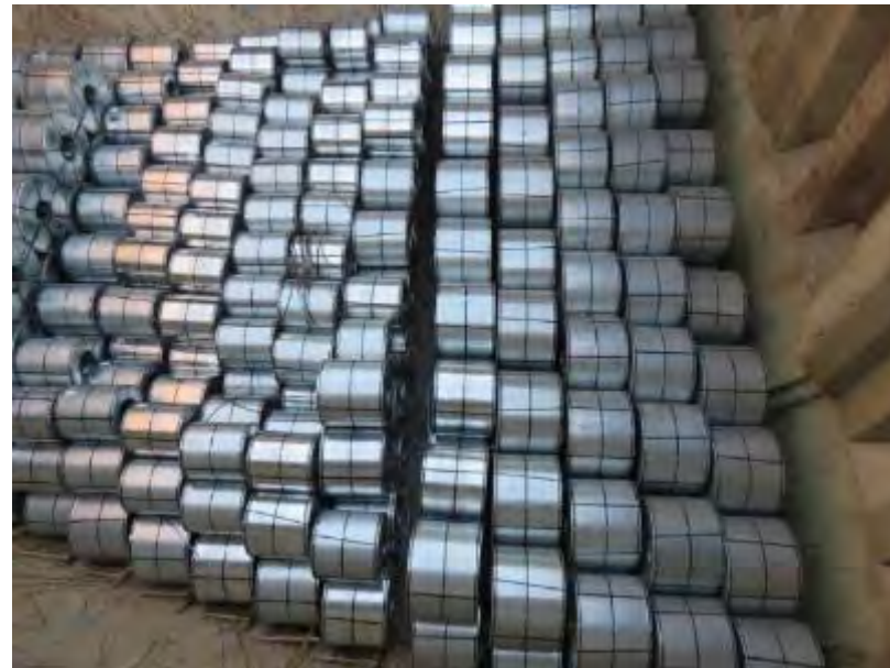
Compact stow of CRCs in a hopper-type cargo hold.
