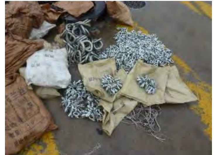
Bulldog grips and additional 'D' rings for cargo lashings.
