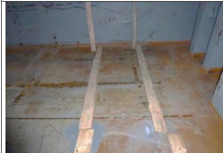
Dunnage in preparation for the loading of coils.
