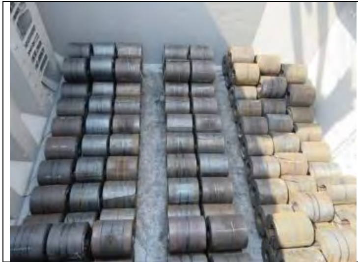
Homogeneous stow of HRCs prior to the lashing. Sufficient space between the rows allowing for the slings to be passed through the coils.
