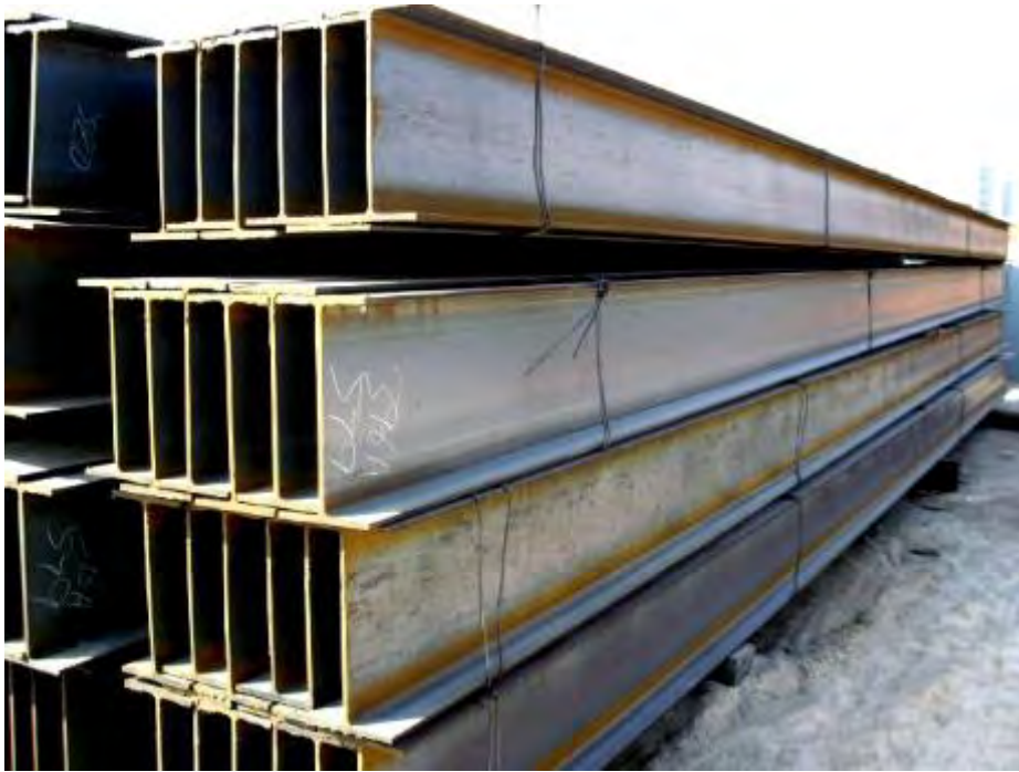
Units in open storage prior to shipment, showing signs of corrosion.
