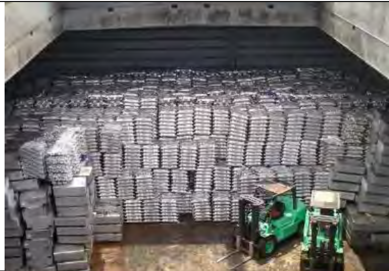
Use of forklift trucks for off-loading bundled ingots and T-ingots from a box-type cargo compartment.
