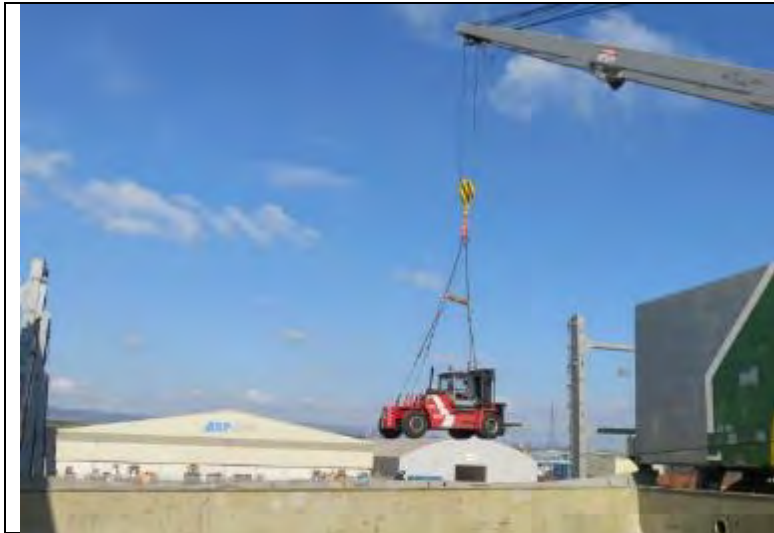
Lowering of a forklift truck in the cargo hold for stowing the coils.
