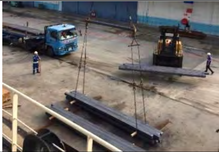
Off-loading blooms with the use of a single chain-leg basket lift under a spreader.
