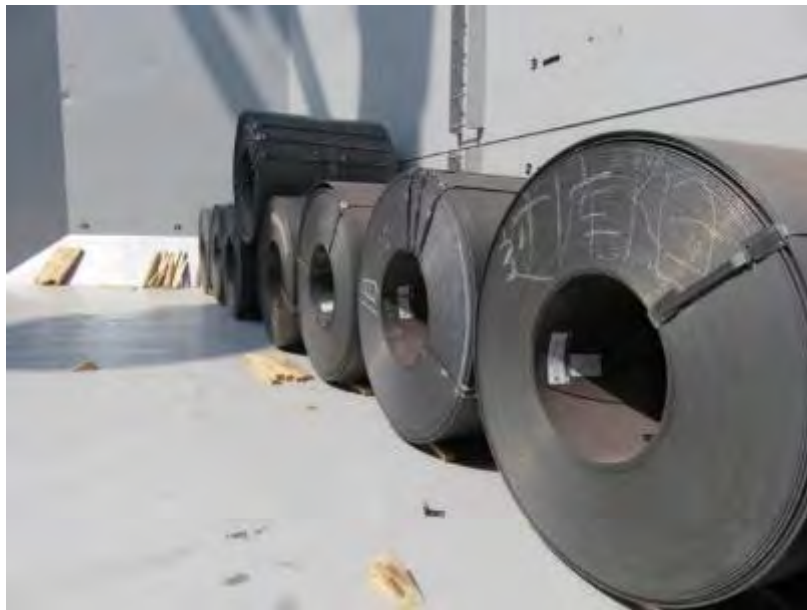
Hot Rolled Steel Coils with insufficient metal straps shall not be accepted for loading.
