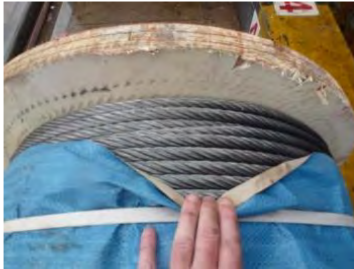
16mm wire rope supplied for lashing cargo.
