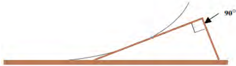
Correct use of the wedge with the right angle on top.
