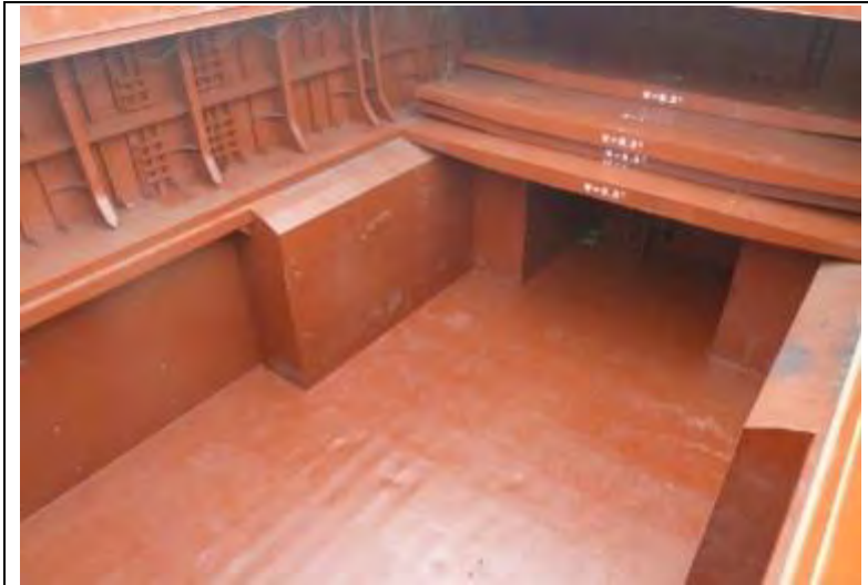
A cargo ship with box-shaped cargo holds and pontoon 'tween deck ready for loading.
