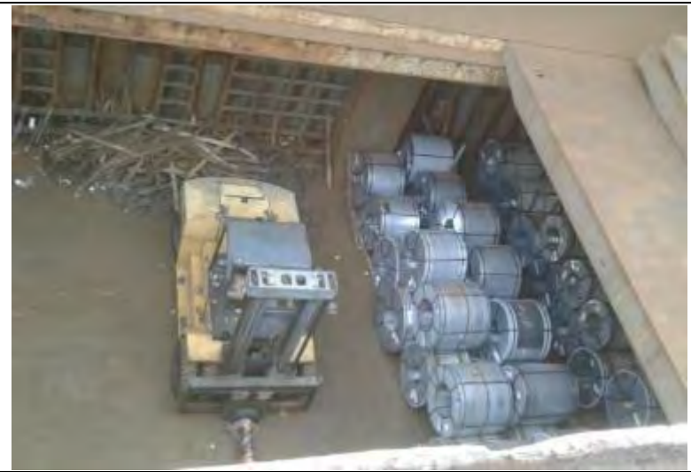
Use of a forklift truck, equipped with a pole to handle the coils under the coaming area.
