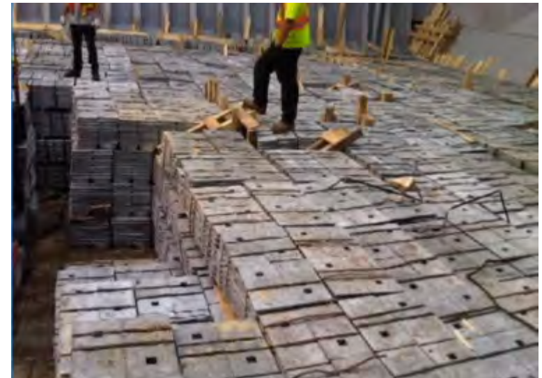
A full stow of small-size ingots in bundles. Choking dunnage used in the stow, and shoring dunnage used against the bulkheads.
