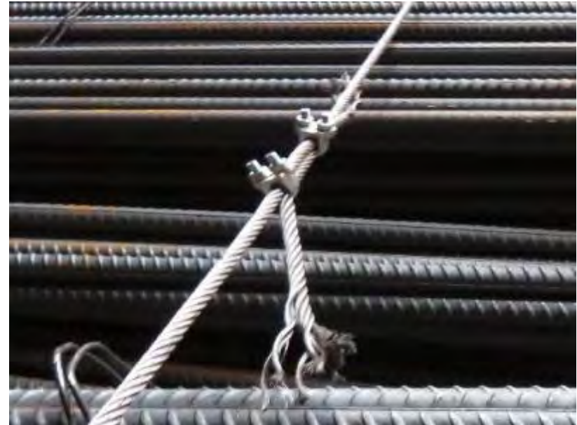
Correct way of using bulldog grips with grips on the live wire. Insufficient number of grips used.
