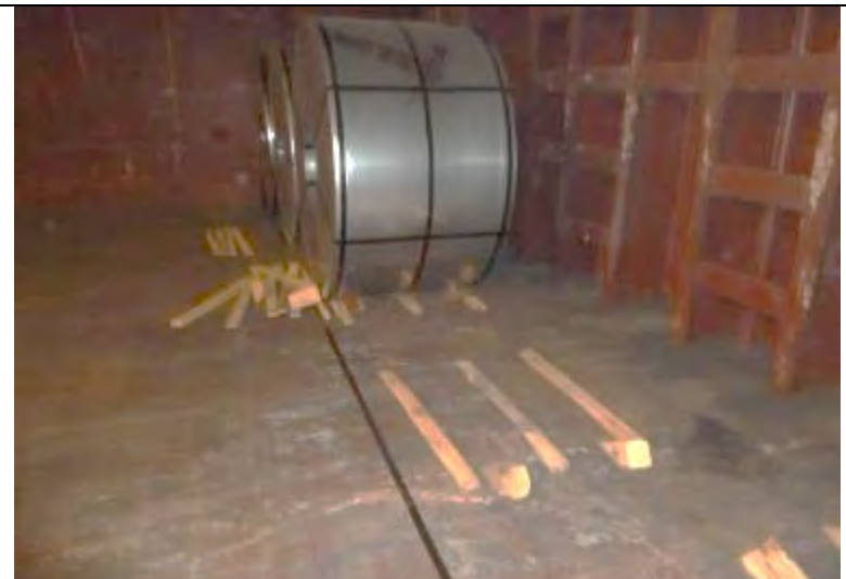
Dunnage in preparation for the loading of coils.
