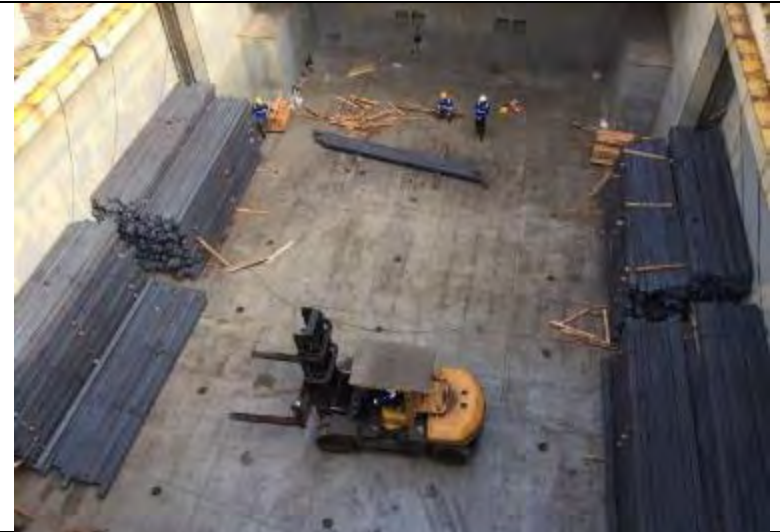
Handling of blooms inside the cargo compartment in preparation for off-loading.
