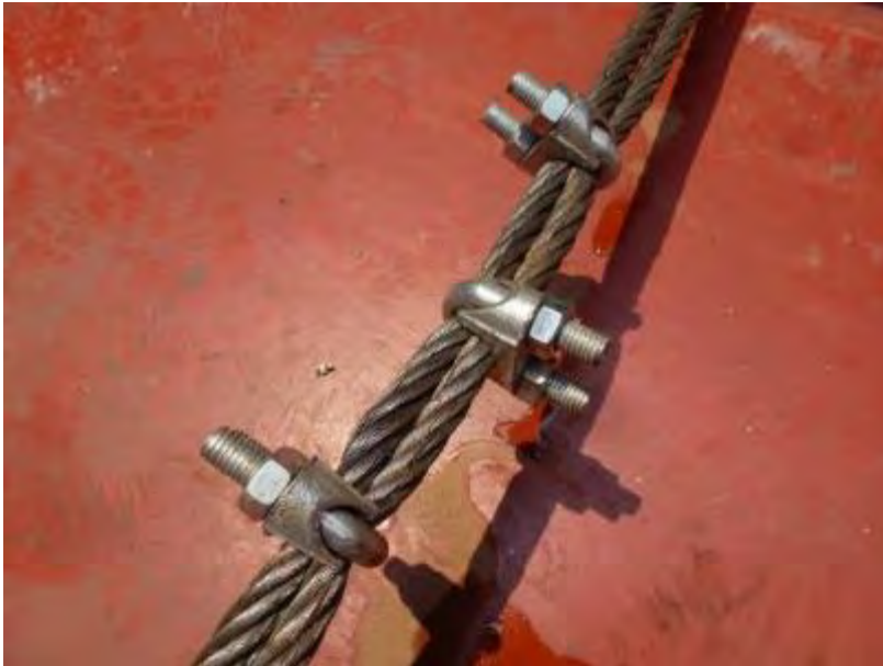
Incorrect way of using bulldog grips.
