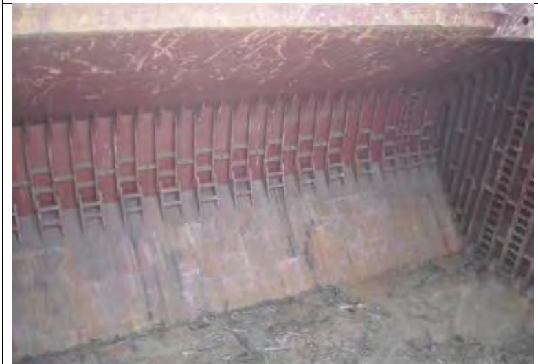
Unprepared cargo hold on a bulk carrier. Residue from some cargoes can react with, and damage, the steel cargo.
