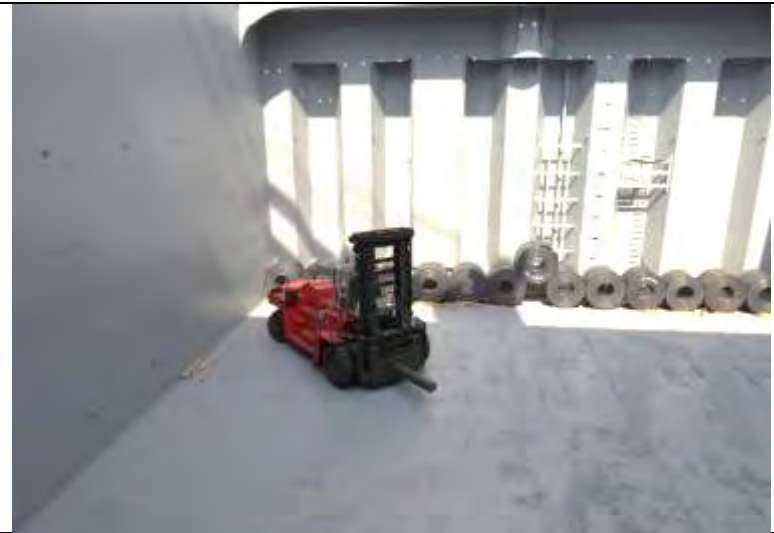
Use of forklift truck with a pole to stow the coils.
