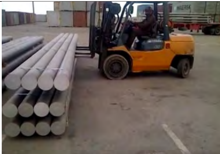
Bundled, long round aluminium billets handled with forklift truck and prepared for loading.
