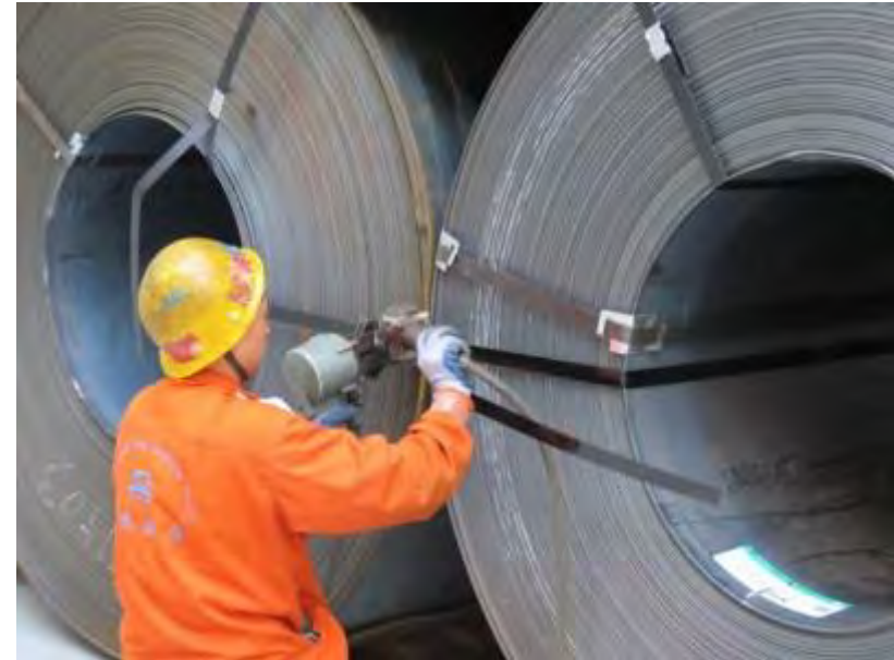
Tightening of steel strapping bands with a pneumatic tool. For coils of the size in the photograph, double metal straps shall be used for lashing.
