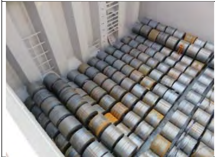
Box-type cargo compartment. A single-tier stow of HRCs without locking coils. The second tier is not complete.
