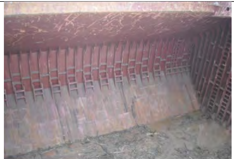
Poorly prepared cargo hold. Again, the cargo residues may react with, and damage, the steel cargo.
