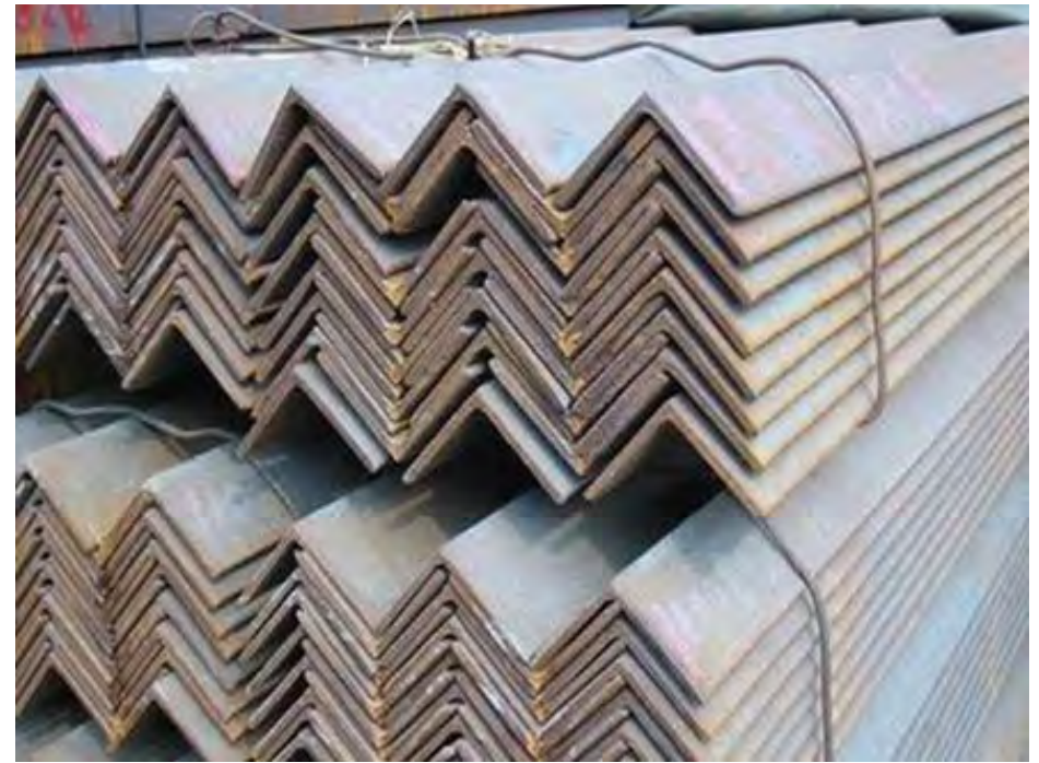
Wire strapping angles along the length of the bundles are not designed for lifting.
