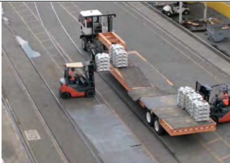
Handling pre-slung, bundled medium-size ingots. Loading on a trailer for further storage in a warehouse.
