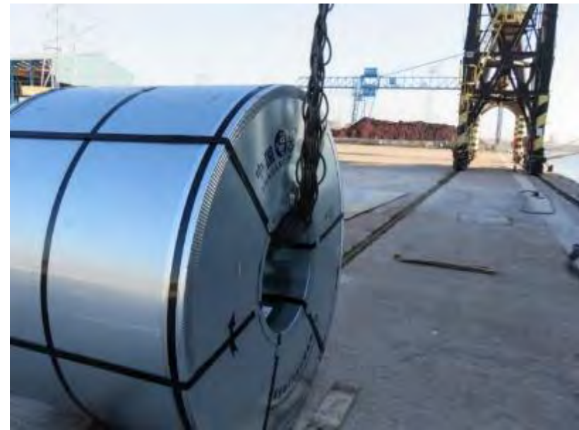
Packaged Cold Rolled Steel Coil off-loaded with braided sling.
